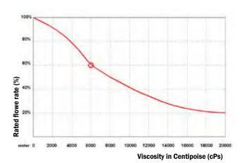
During the delivery of a fluid with a viscosity of 6000cPs, the pump rate decreases to 60% of its rated value (100% = water). Valid for 3/4" pumps & larger.
